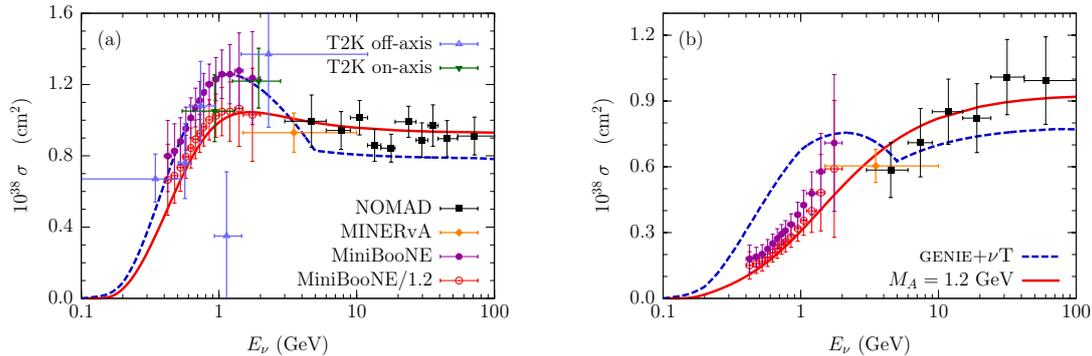
**Figure 5.6:** CCQE (a)  $\nu_\mu$  and (b)  $\bar{\nu}_\mu$  cross sections. The results for carbon obtained using GENIE +  $\nu T$  (dashed lines) and the Spectral Function approach with  $M_A = 1.2$  GeV (solid line) are compared with the carbon data reported by the MiniBooNE [40, 41] and NOMAD [103] Collaborations and the hydrocarbon data extracted from the MINERvA [44, 142] and T2K [139, 143] experiments. For comparison, the MiniBooNE data divided by 1.2 are also shown.
