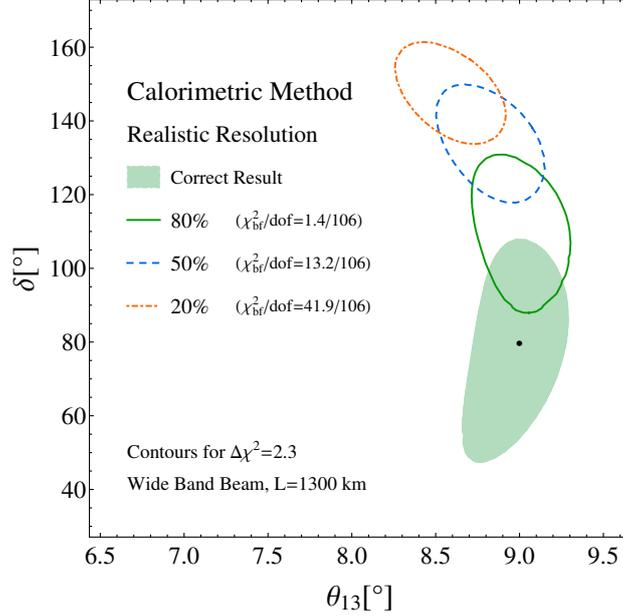
**Figure 5.5:** Effect of an underestimation of the missing energy in the calorimetric energy reconstruction on the confidence regions in the  $(\theta_{13}, \delta)$  plane, see text for details. The true values of the oscillation parameters are indicated by the dot, and are the same for all contours shown.
