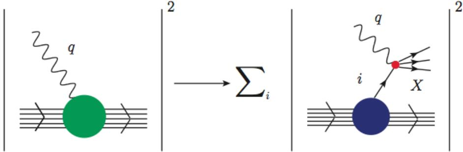
**Figure 3.1:** Schematic representation of lepton-nucleus scattering within the IA. The nuclear cross section is described as the incoherent sum of the elementary processes off the nucleons, and the residual system of  $(A - 1)$ -nucleons acts as spectator.
