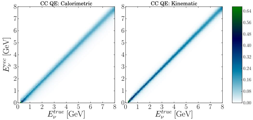
**Figure E.1:** Migration matrices obtained with calorimetric (left panel) and kinematic (right panel) reconstruction. The events in the QE interaction channel, produced with GENIE, are reconstructed using the realistic scenario.
