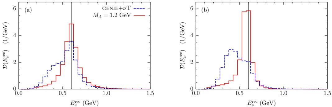
**Figure 5.9:** Reconstructed energy distributions of CC QE (a)  $\nu_\mu$  and (b)  $\bar{\nu}_\mu$  events with any number of nucleons calculated at  $E_\nu = 0.6$  GeV. The dashed (solid) lines represent the results obtained using the GENIE +  $\nu T$  (effective) approach.
