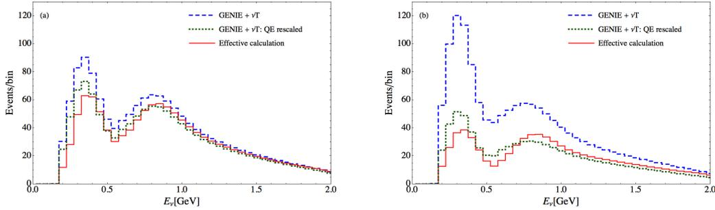
**Figure 5.8:** Distribution of CC (a)  $\nu_\mu$  and (b)  $\bar{\nu}_\mu$  events in the far detector as a function of the reconstructed energy, obtained within the GENIE +  $\nu T$  and effective calculations. For comparison, we also show the GENIE +  $\nu T$  results with the unoscillated QE event rates rescaled to those of the effective calculations.
