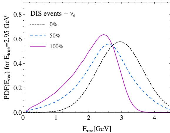
**Figure 5.4:** Reconstructed energy distributions obtained for  $\nu_e$  deep-inelastic scattering (DIS) events with true energy of 2.95 GeV. The distributions neglecting the shift due to the missing energy (dot-dashed line), and accounting for its 50% (dashed line) are compared to the full calculations (solid line).
