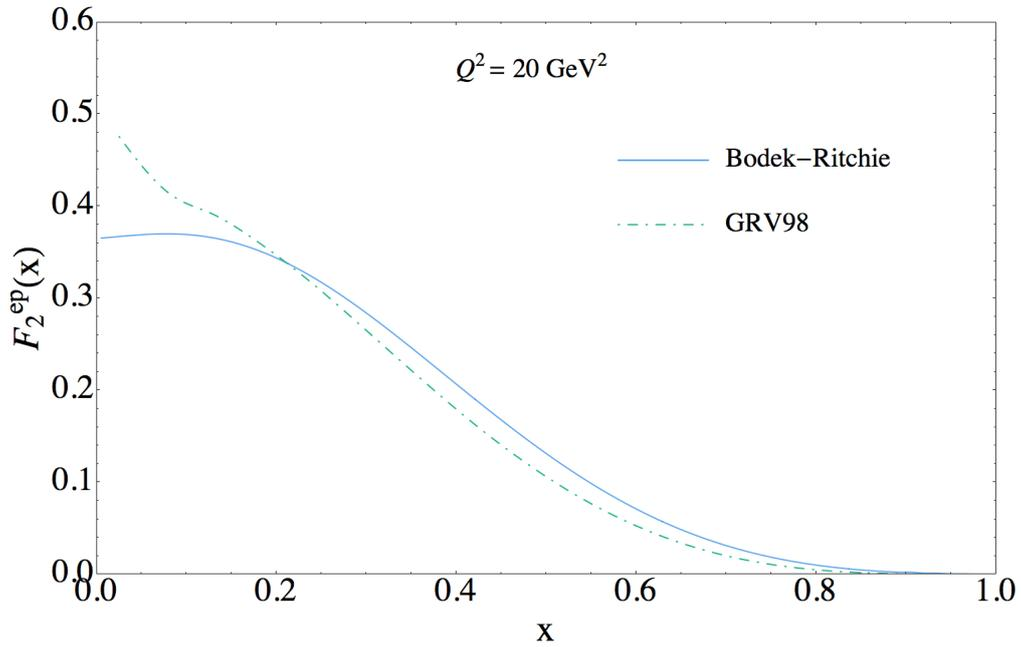
**Figure 2.4:** Behavior of the proton structure function  $F_2^{ep}$  at  $Q^2 = 20 \text{ GeV}^2$ , obtained using the Bodek and Ritchie parametrization (solid line) and the GRV98 parametrization (dot-dashed line). In the second case the structure function is computed using PDFs.
