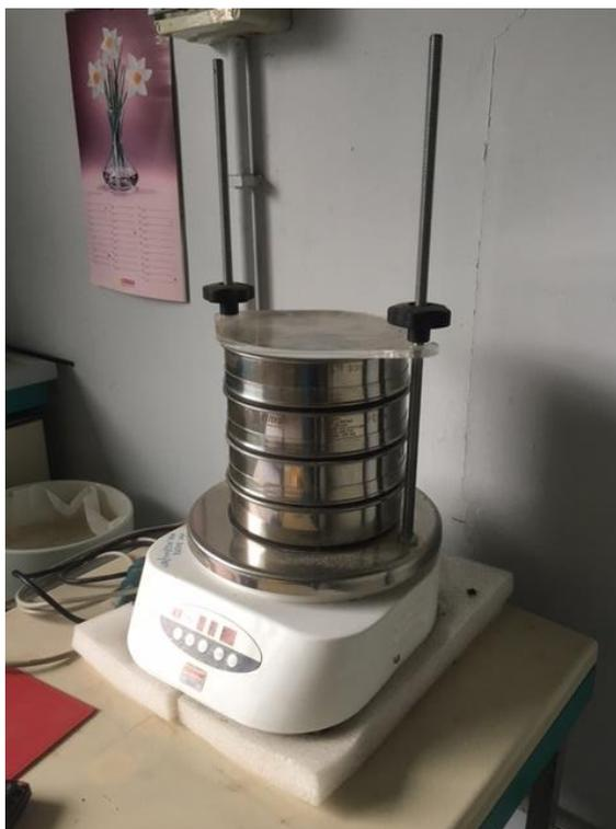
Figure 3.4. Device used to sift the Tuff powder.
