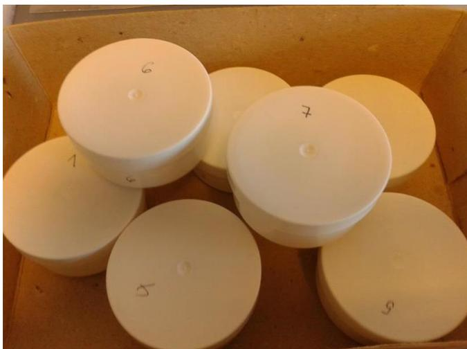
Figure 3.14. Seven identical containers filled with the same amount of Ionex resin.
