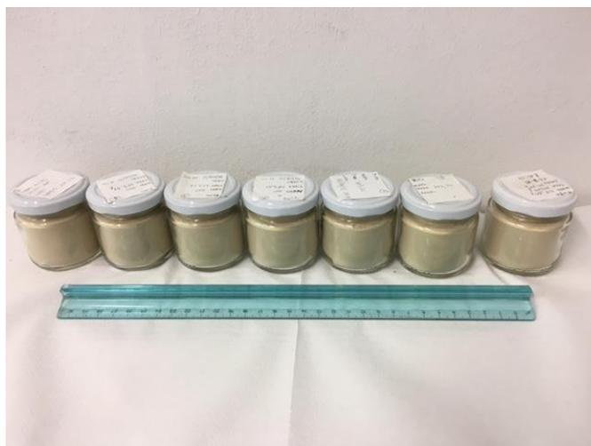
Figure 3.13. Tuff sample used for homogeneity evaluation.
