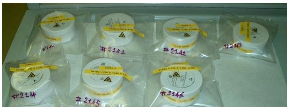
Figure 3.29. The CMR Ionex resin filled in the seven identical containers.
