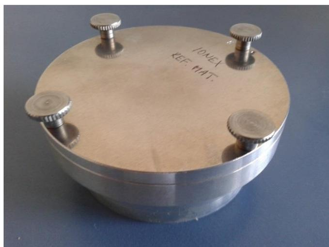
Figure 3.28. The metallic container with Ionex resin sample inside.
