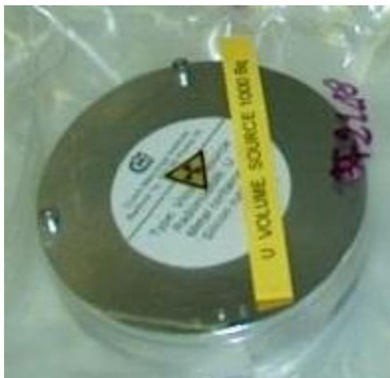
Figure 4.1.  $^{235}\text{U}$  source provided by JRC.
