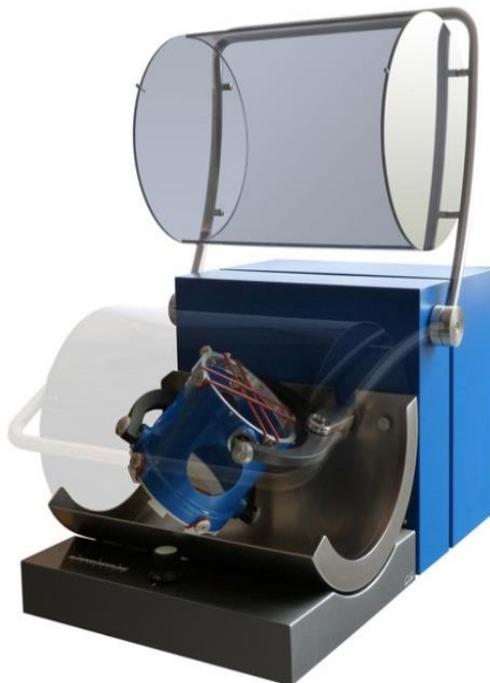
Figure 3.8. Inversina 2 L mixer used to homogenized the powder.
