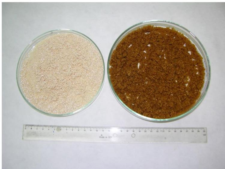
Figure 3.5. Ionex before (right side) and after (left side) regeneration.
