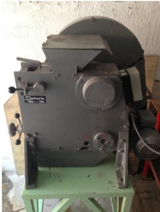
Figure 3.2. Grinder used in the Tuff preparation.
