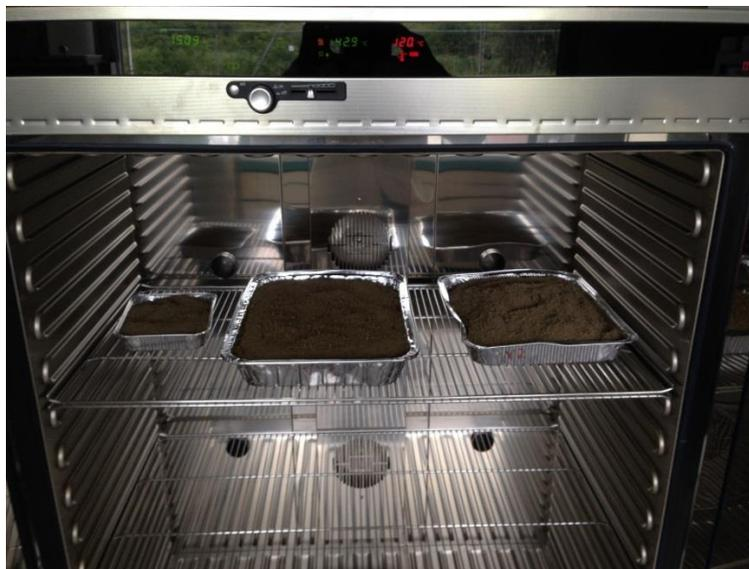
Figure 3.3. Oven used to dry the Tuff sample.
