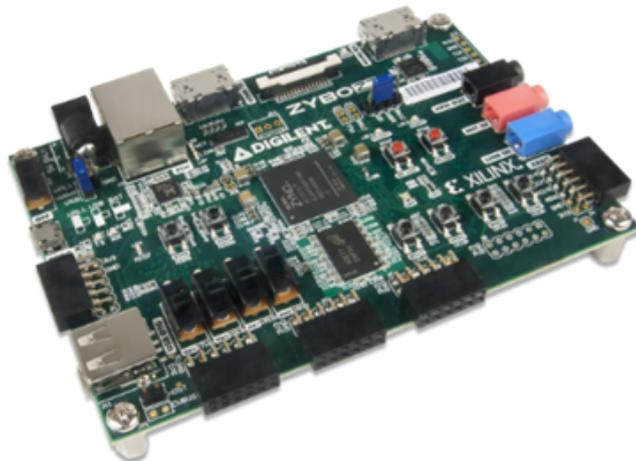
**Figure 2.12:** The Zybo Z7-10 board, from [34]
