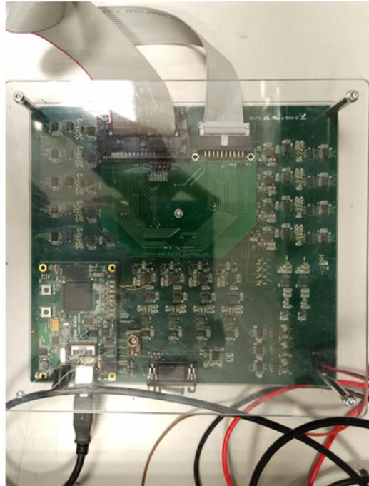
**Figure 2.3:** Control board. The IDC connectors on top bring the power supply to the test board. The USB connector at the bottom gives access to the acquisition software. This board is put outside the irradiation rooms.
