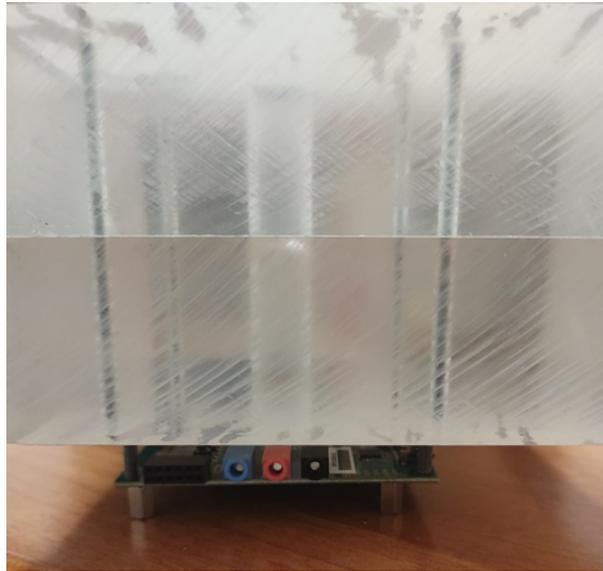
**Figure 4.3:** Image of the Zybo Z7-10 board shielded by a 8 cm plastic shield. The column in the centre is a hole dug aimed to let the beam interact with the electronics involved in the computations related to the network.
