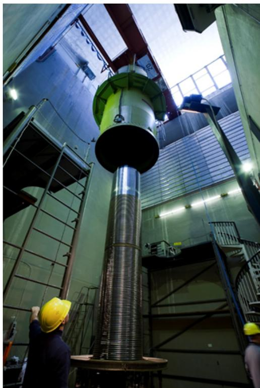
**Figure 4.1:** Column of the CN accelerator being placed inside the tank, picture taken by Andrea Alessio, from [75].
