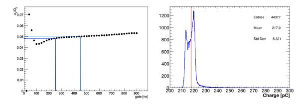
**Figure 6.7:** Left: charge resolution as a function of the integration range of the waveforms due to laser trigger. Right: initial pedestal charge distribution.
