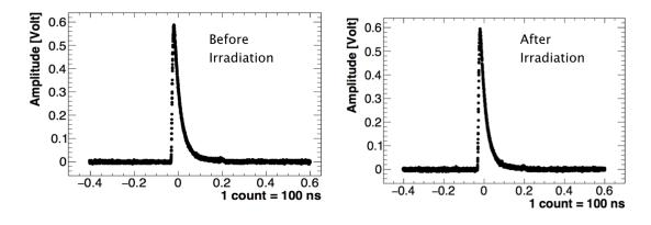
**Figure 5.16:** SiPM digitized waveform when exposed to LED light before (left) and after (right) gamma radiation exposure.
