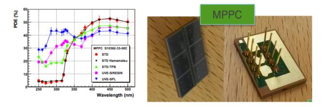
**Figure 3.5:** Left: photodetection efficiency as a function of the wavelength for four SiPM prototypes. The typical PDE values of the standard SiPM S10362-33-50C from Hamamatsu are shown for comparison. These measurements were performed at 25° and include effects of cross-talk and after-pulses. Right: picture of Mu2e array SiPM.
