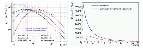
Figure 7.2: Left: fit results to the experimental data: the three dotted lines are the prediction of the standard Gaisser's formula and the solid lines are prediction of the modified formula. Right: generated energy distribution of all the cosmic muons in the horizontal production plane (blue line) and of cosmic muons producing hits in the calorimeter (red line).
