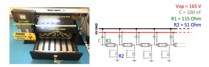
**Figure 4.28:** Left: picture of the RIN station. Right: sketch of the bias and output board for the SiPMs used in the RIN station. A RC filter is placed in the bias pins using R1 and C, while R2 is placed in the output pin.
