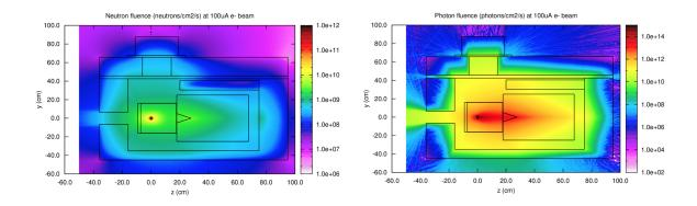
**Figure 5.18:** Distribution of the neutron (left) and of photon (right) fluences as a function of the position around the shielding for an electron current of 100  $\mu$ A.
