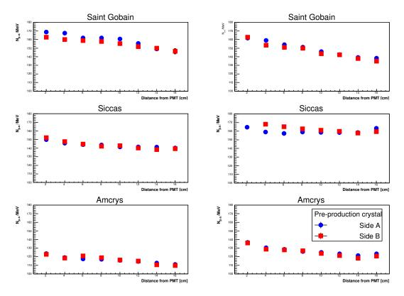
**Figure 4.12:** Example of LRU measurement for 6 different crystals: 2 Sain Gobain cystals (top), 2 from Siccas (middle) and two from Amcrys (bottom). Blu points are taken with the PMT coupled with A side, red squares with B side.
