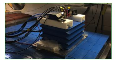
**Figure 5.23:** Experimental setup mounted in EPOS on top of the shielding. The SiPM surface is located at 2.2 cm from the neutron shielding (blue lead blocks) and 90 cm far away from the neutron source.
