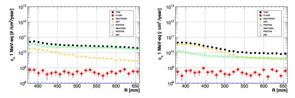
**Figure 3.20:** 1 MeV-equivalent neutron flux as a function of the radial position at the back face of the front (left) and back (right) disk. The backgrounds representing less than 1% of the total flux are not drawn.
