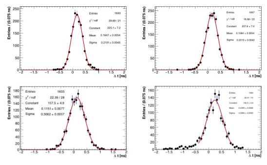
**Figure 6.25:** Time resolution of the crystals readout by AdvanSiD (left) and SensL (right) SiPMs. The top plots are related to the 1 GHz sampling rate, the bottom ones are obtained with the offline resampling at 200 MHz
