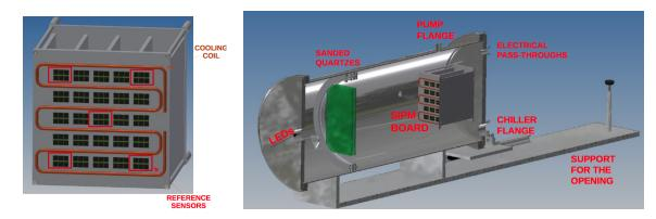
Figure 5.36: CAD drawing of the experimental te
