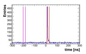
**Figure 5.11:** Time of the detected peaks. The zero corresponds to the LED pulse. The peak between 10 and 30 ns results from the LED light, while the flat background is due to dark pulses.
