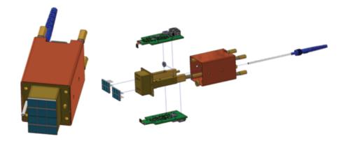
**Figure 3.8:** Left: assembly of the FEE holder. Right: exploded view of the FEE holder with all the components. Two SiPMs glued on the inner cupper support, FEE AMP-HV boards, Faraday cage and needle for insertion of the optical fiber.
