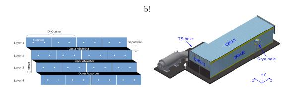
**Figure 2.13:** Left: the CRV system is an active veto made by a system of four layers of long scintillator strips, with an aluminum layer between them. Right: the cosmic ray veto covering the Detector Solenoid and half of the Transport Solenoid.
