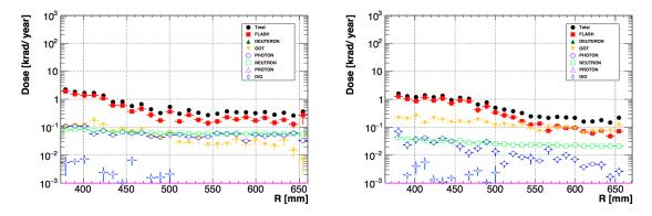
**Figure 3.19:** Expected dose in the front (left) and back (right) CsI disks as a function the radius where the crystals are located.
