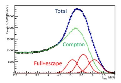
**Figure 3.14:** Energy spectrum for a crystal irradiated with 6.13 MeV photons from an  $^{16}O^*$  source.
