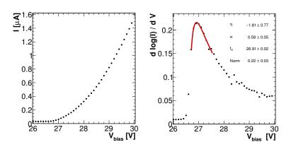
**Figure 5.5:** Left: example of an I-V scan. Right: dark current logarithmic derivative as function of the SiPM bias voltage. The red line represents the log-Gaussian fit used to extrapolate the breakdown voltage as the peak position value.
