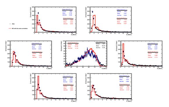
Figure 6.15: Data (black dots)-MC (red line) comparison of the energy deposit in the central crystal and the first surrounding ring
