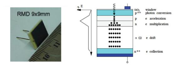
Figure 3.4: Left: picture of an APD sample. Right: Schematic layout of the Avalanche Photodiode. An intrinsic (or lightly doped p-type) material  $\pi$  sandwiched between a heavy doped p-side and a heavy doped n-side. Another p-type region is also established between the intrinsic material and the heavily doped n side. A strong reverse bias between the two ends creates an electric field E.
