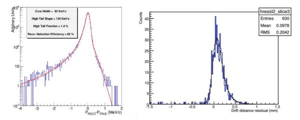
Figure 2.12: Tracker momentum resolution with simulated CEs. Full background overlay and pattern recognition included. Fit to a split double Gaussian with standard track fit quality cuts. The core width satisfies the Mu2e momentum resolution requirements [1].
