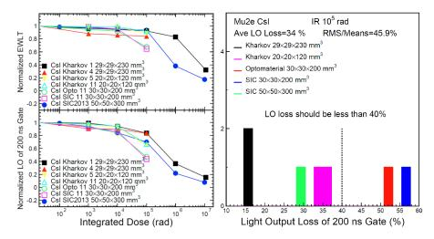
**Figure 4.23:** Left: normalized emission weighted longitudinal transmission (EWLT, top) and light output (LO, bottom) are shown as a function of integrated dose for undoped CsI crystals from various vendors. Right: summary of the normalized light output loss measured in 200 ns integration time for undoped CsI crystals from different vendors after 100 krad.
