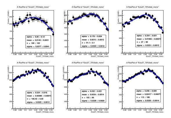
Figure 7.33:  $E_{cluster}/P_{traker}$  distribution obtained at 0.7 T for the six momentum values used in the simulations, as reported in Table.
