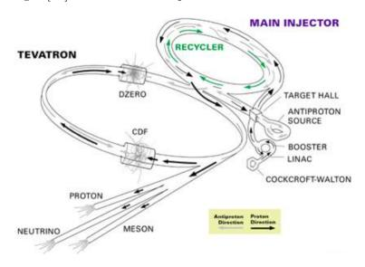
Figure 2.2: Layout of the accelerator complex providing the proton beam to Mu2e. Protons are transported from the Booster through the MI-8 beamline to the Recycler Ring where they will circulate while they are re-bunched by a 2.5 MHz RF system. The reformatted bunches are kicked into the P1 line and transported to the Delivery Ring where they are slow extracted to the Mu2e detector through a new external beamline.
