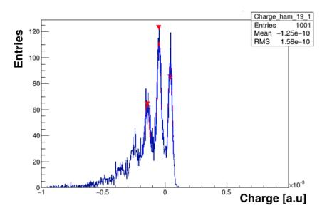
**Figure 5.8:** Charge distribution distribution for a SiPM's cell illuminated by a LED light. Red markers indicate the distribution's peaks. That Gain is evaluated using the peaks distance.
