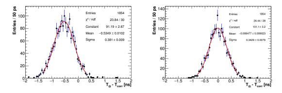
**Figure 7.10:** Distribution of the fit residuals for a single crystal at the first iteration (left) and after 5 iterations (right) considering all the calibration sample. A gaussian fit is performed to determine the corresponding  $T_{0i}$  value.
