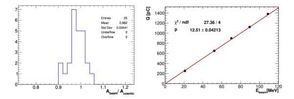
**Figure 6.14:** Left: Ratio of Ai factors for beam and cosmic calibration techniques. Right: mean value of the charge reconstructed at different beam energy as a function of the expected energy deposit at different beam energy.
