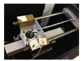
**Figure 4.8:** Left: efficiency curve of the UV-extended photomultiplier tube used for the measurements. Right: detail of the setup used to test crystals. The coupling of a wrapped crystal with the PMT is visible. The cart bringing the source is also visible.
