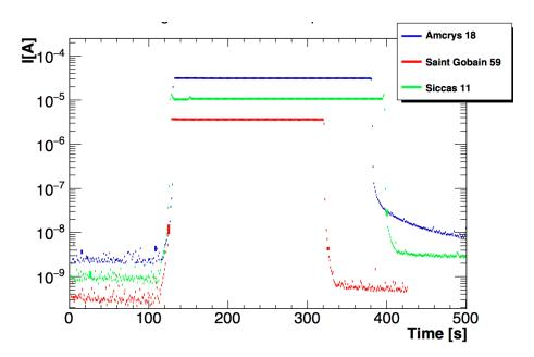
**Figure 4.18:** Example of RIN measurement for a SICCAS (green), Amcrys (blue) and Saint Gobain (red) crystal. The photocurrent plateau occurs when the  $^{137}Cs$  source cart is over the crystal.
