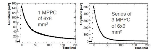
**Figure 5.2:** Left: digitized waveform of a single  $6 \times 6$  mm<sup>2</sup> SiPM cell. Right: digitized waveform of a series of three  $6 \times 6$  mm<sup>2</sup> SiPM cells.
