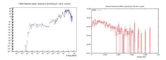
Figure 5.19: 1 MeV equivalent neutron (left) and gamma (right) spectra for an electron current of 1  $\mu$ A at the SiPMs position.
