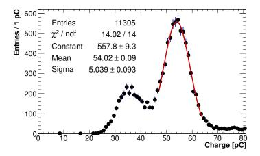
Figure 4.10: Charge distribution of the LYSO-tag system. The distribution red fit is a gaussian function used to evaluate the mean value and the  $\sigma$  of the distribution. Events are selected only if their peak time is around  $\pm 2\,\sigma$  of the mean value.
