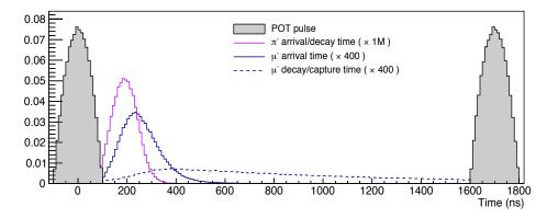
Figure 2.5: The proton beam hits the production target with bursts 200 ns large and separated from the next one by  $\sim 1700$  ns. The detector system starts taking data after 670 ns from the arrival of the proton pulse, when almost all pions are decayed. Muon capture time in Al (dashed blue line) best matches this timing scheme.
