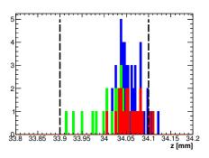
**Figure 4.3:** Stack distribution of the transverse dimensions along the horizontal (left) and vertical (right) axis with respect to the measurement table of the CMM. Black dashed lines shows the limits imposed by the mechanical requirements.
