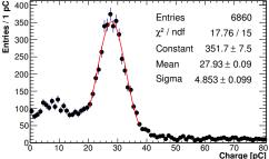
Figure 4.11: Left: Time distribution mean value, fitted with a gaussian function to evaluate the mean value and the  $\sigma$  of the distribution. Events are selected only if their peak time is around  $\pm 3 \sigma$  of the mean value. Right: Charge distribution of the crystal under test after the timing selection and the TAG charge cuts.
