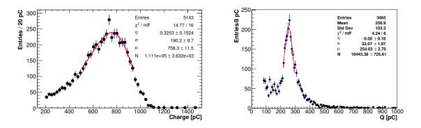
Figure 6.13: Charge deposited by 100 MeV electron beam (left) and cosmic (right) events.
