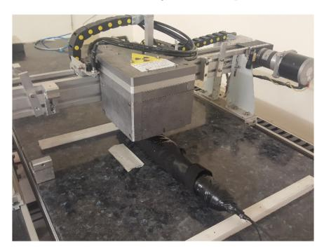
Figure 4.17: Experimental apparatus for RIN measurements: a motorized cart transport a strong  $^{137}Cs$  source over the CUT.
