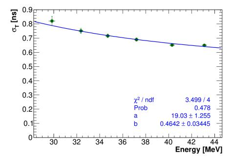
**Figure 7.41:** Time resolution as a function of the deposited energy obtained for the most energetic neighbouring crystals when the beam impinges at 50 degrees the Module-0.
