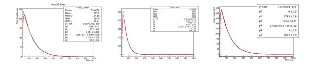
**Figure 5.15:** Average waveform for a single cell of the AdvanSiD (left), Hamamatsu (middle) and SensL (right) SiPM.
