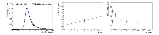
Figure 3.18: Left: energy resolution fit with a double-sided Crystal Ball function, quoting both core resolution ( $\sigma$ ) and FHWM/2.35. The core resolution is more sensitive to the pile-up, while the FHWM is more representative of the "total" resolution. Middle: FHWM/2.35 as a function of crystal longitudinal response uniformity. Right: FHWM/2.35 as a function of crystal lyght yield
