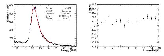
**Figure 7.16:** Left: example of energy distribution obtained after MC-based calibration. The peak due to CR events is fit with a Landau function. Right: MPV values obtained from the Landau fit on all the channels energy distributions.
