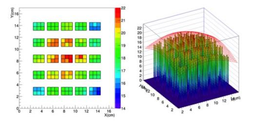
Figure 5.39: LED light intensity reaching the sensors under test.
