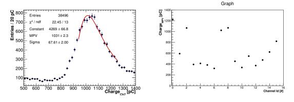
**Figure 7.15:** Left: example of the charge distribution reconstructed by a SiPM of the central channel. The peak due to CR events is clearly visible and fit with a Landau function. Right: MPV values obtained from the Landau fit on all the channels charge distributions.
