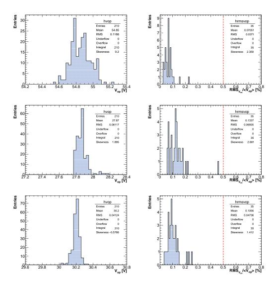
**Figure 5.6:** Left: Distribution of  $V_{op} = V_{br} + 3$  V for all the measured cells of the SiPM from Hamamatsu (top), SensL (middle) and AdvanSiD (bottom) vendors. Right: Distribution of the RMS mean value of  $V_{op}$  among each Mu2e-SiPM cell.
