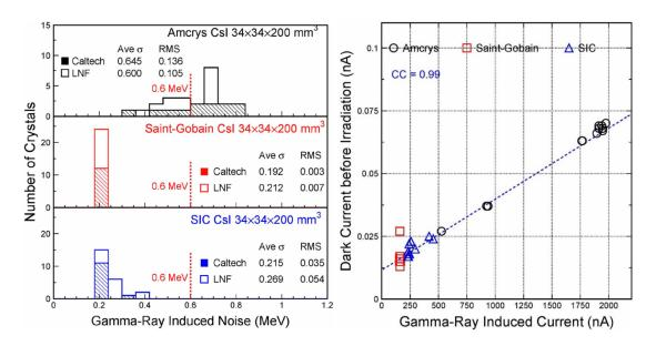
**Figure 4.19:** Left: results of RIN measurements performed on all the 72 pre-production crystals form Amcrys (top), Saint-Gobain (middle) and SICCAS (bottom). Right: dark current before the irradiation as a function of the dark current measured during crystal exposure.
