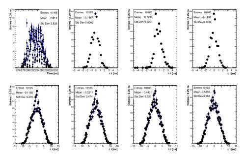
Figure 7.37: Top left: time distribution of the trigger signal of the first chip of the first digitizer board, which is the reference signal. The other distributions on top (bottom) are the time differences between the trigger time of the other DRS4 chips of the first (second) board and the reference.
