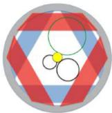
Figure 2.10: Left: The Mu2e straw tube tracker. The straws are oriented transverse to the solenoid axis. Right: cross sectional view of the Mu2e tracker station with the trajectories of a 105 MeV CE (top) and a 53 MeV Michel electron (lower right) superimposed. The disk in the center is the stopping target. Electrons with energies smaller than 53 MeV (lower left) miss the tracker entirely.
