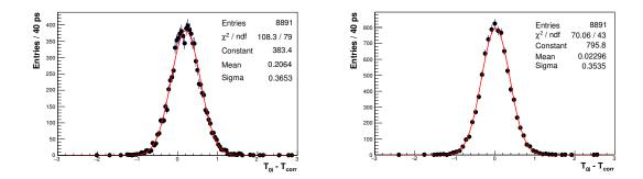
Figure 7.24: Distribution of the fit residuals for a single crystal at the first iteration (left) and after 5 iterations (right). A gaussian fit is performed to determine the corresponding  $T_{0i}$  value.
