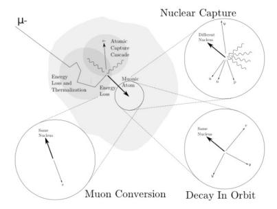
Figure 1.10: A muon stopped in the aluminum target can be captured in an atomic excited state and promptly fall to the ground state. For aluminum, in addition to the electron conversion process,  $\sim 39\%$  of the muons will decay in orbit, while the remaining  $\sim 61\%$  will be captured on the nucleus, producing electrons, photons and neutrons from the atomic cascade.
