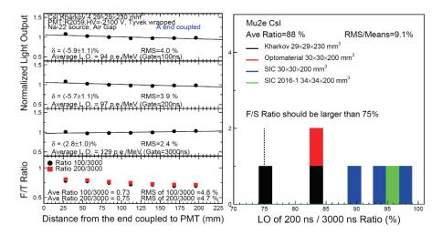
**Figure 4.6:** Left: CsI LRU (top three) measured with 100, 200 and 3000 ns integration gates respectively, and the F/T ratio (bottom) of LO(100 ns) and LO(200 ns) versus LO(3000 ns). Right: Summary of the F/T ratio of LO(200 ns)/LO(3000 ns).
