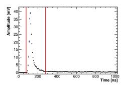
**Figure 4.9:** Left: Digitized waveform of the LYSO tag system. Right: Digitized waveform produced by the 511 keV photon in the pure CsI crystal. The red lines represent the integration range.
