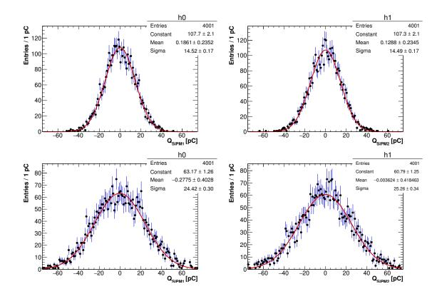
Figure 5.32: Noise distribution of the two Hamamtsu SiPM of the central module-0 channel when illuminated by ambient light, used to simulate the neutron noise and corresponding to a dark current measurement of 500  $\mu$ A (top) and 1500  $\mu$ A (bottom).
