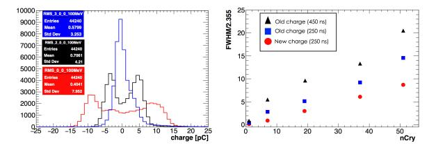
Figure 6.10: Left: Pedestal charge distribution evaluated in 450 ns wf integration range without corrections (black), in the 250 ns range with the linear fit correction (red), in the 250 ns integration range and with the 2-functions based correction (blue). Right: dependence of the RMS of the distribution of the pedestals sum obtained summing up several channels as a function of the number of channels for the three different evaluated charges.
