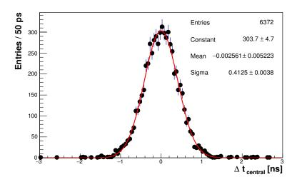
Figure 7.22: Time resolution of the central channel.
