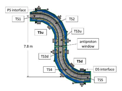
Figure 2.7: Trasnsport Solenoid schematic drawing.
