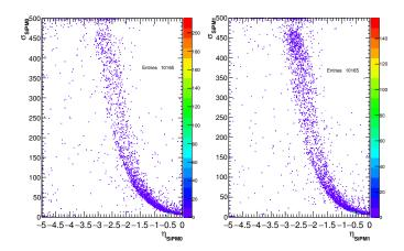
Figure 6.21: Asymmetric parameter  $\eta$  of the log-Normal function as a function of  $\sigma$ , both obtained applying the log-Normal fit on the 200 MHz re-sampled waveforms. A dependance is clearly visible and well represented by a second order polinomial function.
