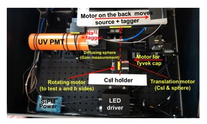
Figure 4.26: Layout of the QA optical automatized station.
