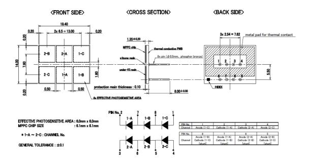
Figure 5.1: Sketch a of the custom Mu2e SiPM array.
