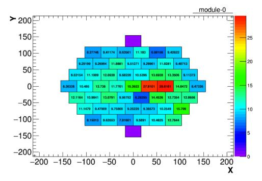
Figure 7.39: Module-0 energy map when a 100 MeV electron beam impinges at 50 degrees.
