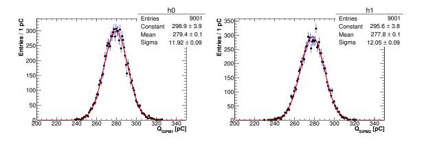
**Figure 5.30:** Charge distribution of the two Hamamtsu SiPM of the central module-0 channel when illuminated by LED light.
