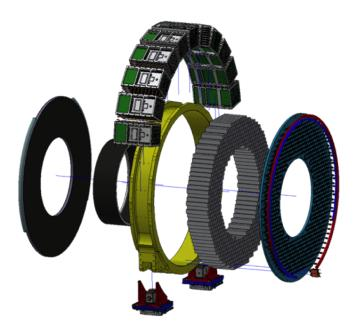
Figure 3.11: Exploded view of the components of the Mu2e calorimeter annular disks.
