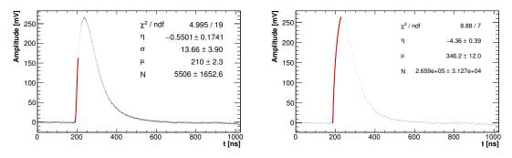
**Figure 6.19:** Example of the outcome of the optimized fit to a waveform at 1 Ghz sampling rate (left) and 200 MHz (right).
