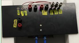
**Figure 5.22:** Pictures of the front (left) and back (right) side of the experimental setup used for SiPMs irradiation test at EPOS facility of HZDR. The three SiPMs under test are covered by black tape to make them light tight and to not disturb the measurement of dark current.
