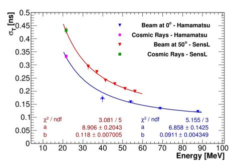
Figure 6.26: Time resolution as a function of the deposited energy in the highest energetic crystal.
