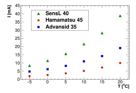
Figure 5.26: Cells current as a function of the temperature at the operational voltage.
