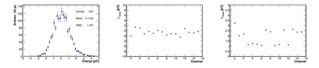
Figure 7.18: Left: example of charge distribution obtained during the pedestal run. Middle: peaks of the noise distributions of all the 16 channels obtained from a gaussian fit. Right: sigma of the noise distributions of all the 16 channels obtained from the gaussian fit.
