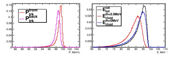
**Figure 7.35:** Left: distribution of the momentum at the beginning and at the end of tracker, for a generated momentum value of 100 MeV. Right: energy reconstructed by the calorimeter considering three different clustering threshold considering a generated momentum value of 100 MeV.
