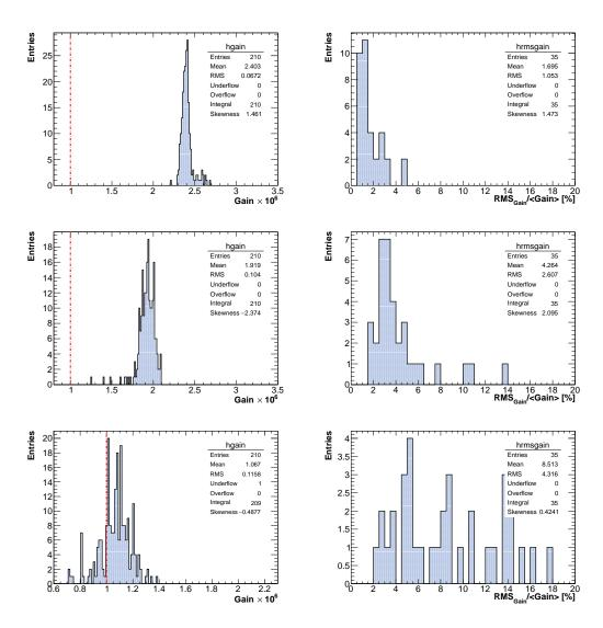
**Figure 5.9:** Left: Distribution of the gain, G, for all sensors in the prototypes batch from Hamamatsu (top), SensL (middle) and AdvanSiD (bottom) vendors. Right: Distribution of the relative gain RMS in each sensor.
