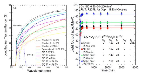
Figure 4.5: CsI EWLT (left) and light output (right).
