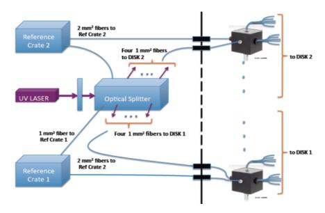
Figure 3.15: Schematics of the Laser Monitoring System.
