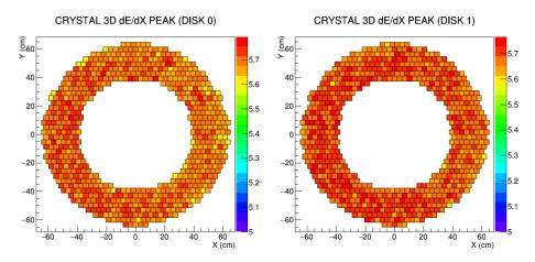
Figure 7.6: 3D specific energy loss in the crystals of the front (left) and back (right) calorimeter disks obtained by the MC simulation.
