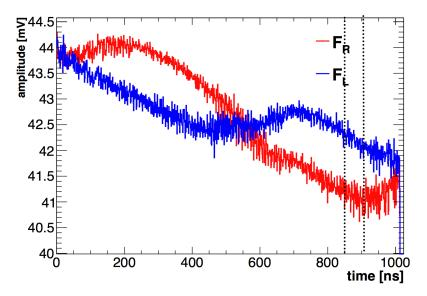
Figure 6.8: Correction functions used to correct the pedestals.
