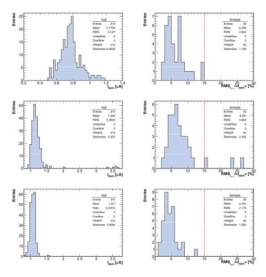
Figure 5.7: Distribution of  $I_{dark}$  (left) and distribution of the RMS mean value of  $I_{dark}$  (right) within each sensor cell from Hamamatsu (top), SensL (middle) and AdvanSiD (bottom) vendors.
