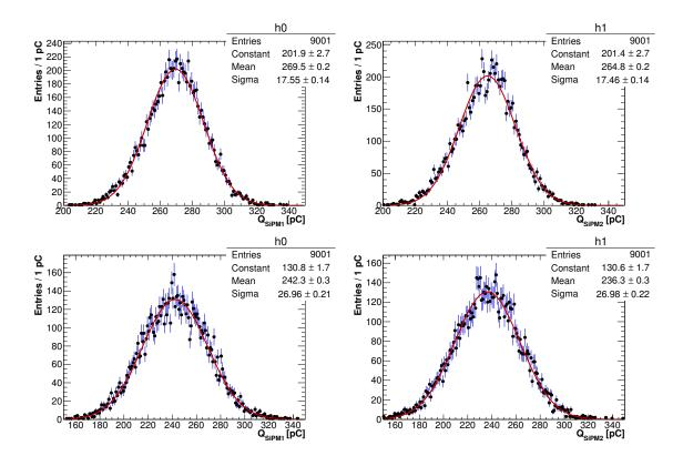
Figure 5.31: Charge distribution of the two Hamamtsu SiPM of the central module-0 channel when illuminated by LED light and ambient light, corresponding to a dark current measurement of 500  $\mu$ A (top) and 1500  $\mu$ A (bottom).
