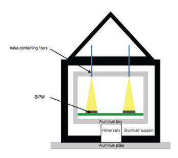
Figure 5.33: Sketch of the box used for the MTTF SiPMs test.
