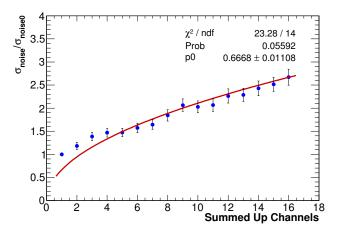
Figure 7.19: Noise value obtained summing up several channels noise as a function of the number of channels
