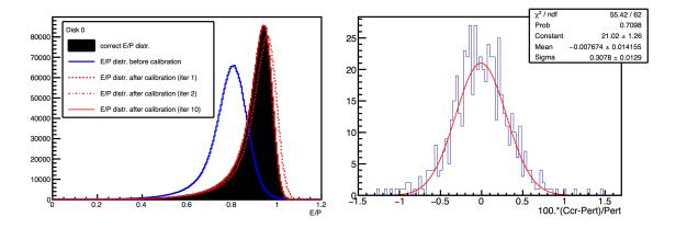
Figure 7.32: Left: distribution of the cluster energy, E, and tracker momentum measurement, P, ratio. Right: distribution of the difference between the iterative calibration constant and the perturbation coefficient,  $\lambda_i$ , normalized to  $\lambda_i$ .
