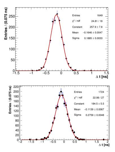
**Figure 6.23:** Time resolution of the central crystal readout by two Hamamatsu SiPM with a beam energy of 100 MeV. On left the sampling rate is at 1 GHz, on right the waveform has been resampled offline at 200 MHz. The red lines represent the Gaussian fit performed.
