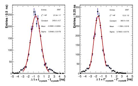
**Figure 7.40:** Time difference between crystal A and B before (after) trigger time correction on left (right).
