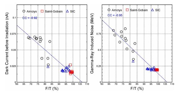
**Figure 4.20:** Dark current before the irradiation (left) and  $\gamma$ -RIN (right) measurements as a function of the F/T ratio.
