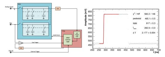
**Figure 7.36:** Left: Trigger scheme of the DRS4 chip used in the V1742 CAEN digitizer board. Right: NIM trigger signal digitized at 1 GHz sampling rate. The red line represents the fit used to evaluate the signal time.
