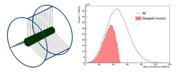
**Figure 2.9:** Left: schematic layout of the Mu2e stopping target and its mechanical support. It is made by 17 aluminum disks, 0.22 mm thick, spaced 5 cm along the DS axis. The disks radius decreases from 8.3 cm upstream to 6.3 cm downstream. Right: momentum distribution of muons delivered to the stopping target as well as the distribution of muons that stop (red) in the Al foils.
