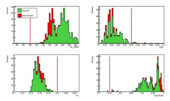
Figure 4.27: Optical properties of the production crystals measured with the automatized station.
