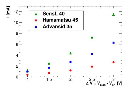
Figure 5.27: Vendor cells current as a function of  $\Delta V$ . Temperature was kept stable at 0 ° C.
