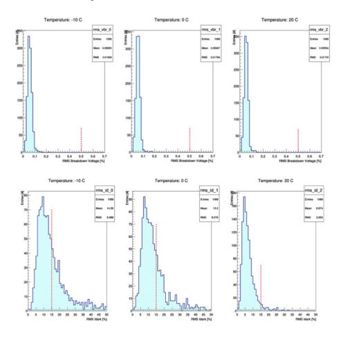
Figure 5.38: Spread on the  $V_{br}$ , on top, and on the  $I_d(\text{at }V_{br})$ , on bottom, measurements performed over the six cells of the Mu2e production SiPMs.
