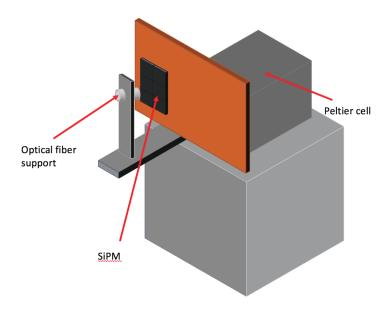
Figure 5.13: Sketch of the experimental setup used for the recovery time measurmenet test.
