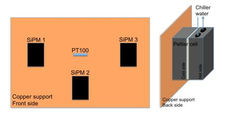
**Figure 5.20:** Front (left) and back (right) sketch of the experimental setup used for SiPMs irradiation test at EPOS facility of HZDR.
