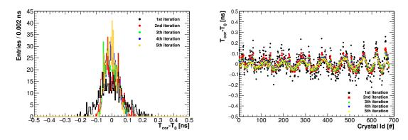
Figure 7.12: Left: difference between the initial  $T_0$  and the correction to be applied at each iteration. Right: same distribution as a function of the crystal id.
