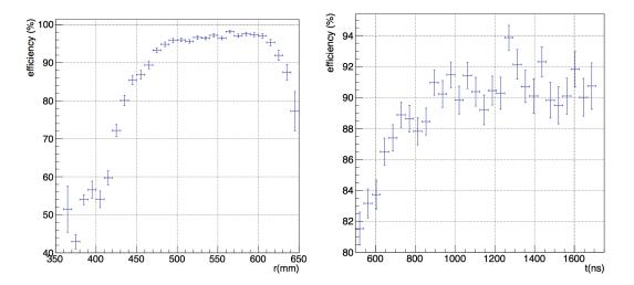
**Figure 3.25:** Left: CE BDT efficiency versus the conversion electron impact radial position after preselection. Right: CE BDT efficiency versus the conversion electron time position after preselection.
