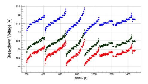
Figure 5.37: Breakdown voltage measured at three different temperature (-10  $^{\circ}$ Cin red, 0  $^{\circ}$ C in green, 20  $^{\circ}$ C in blue) as a function of the SiPM identification number.
