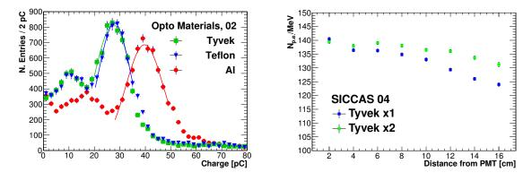
**Figure 4.7:** Left: Reconstructed charge of a CsI crystal from Opto Materials when tested with a  $^{22}$ Na source and wrapped with different materials. Right: light yield of a CsI crystal sample from SICCAS when wrapped with one or two layers of a 150  $\mu$ m tick Tyvek foil.
