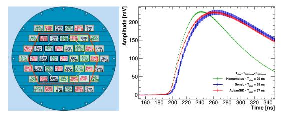
Figure 6.24: Left: Vendor SiPM map in the Module-0. Right: profiles of 1000 normalised waveforms per vendor obtained during the calibration runs done with 100 MeV energy beam impinging orthogonally on each crystal.
