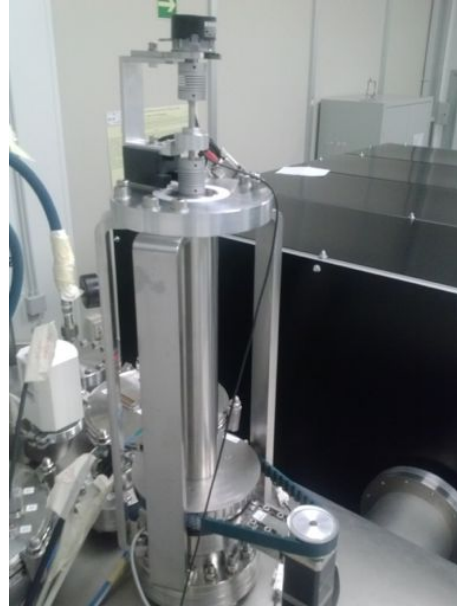
(b) The rotation axis with the potentiometer installed.
