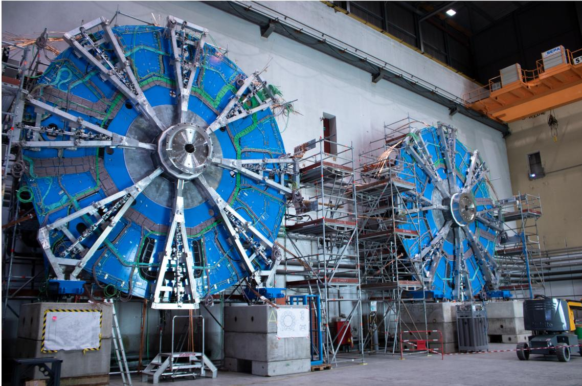
**Figure 3.5:** Images of the two mechanical structures of the ATLAS New Small Wheels ready to host the chambers.
