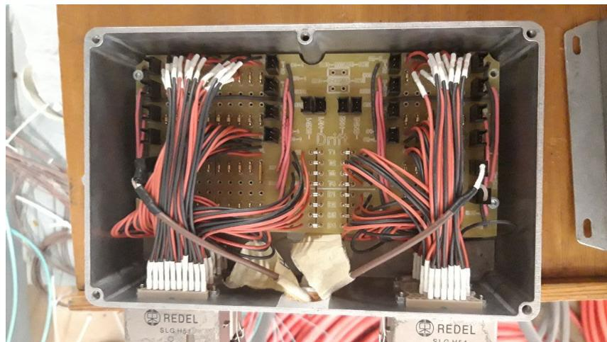
**Figure 3.56:** Picture of the splitter box. The cables coming from each module of the double-wedge are connected to the splitter box as for the cables coming from the high voltage power supply. The gold jumpers are used to connect the sections to their channel.
