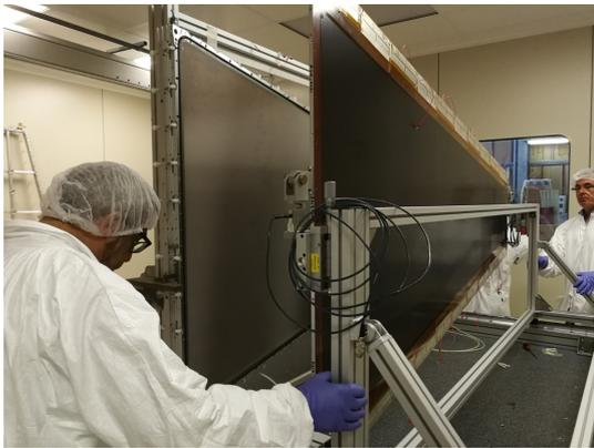
(a) Picture during the closure of the first gas gap of a quadruplet.
