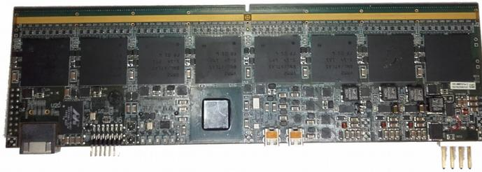
**Figure 3.23:** Picture of a MMFE8 readout board. Eight VMM3a can be seen on top.
