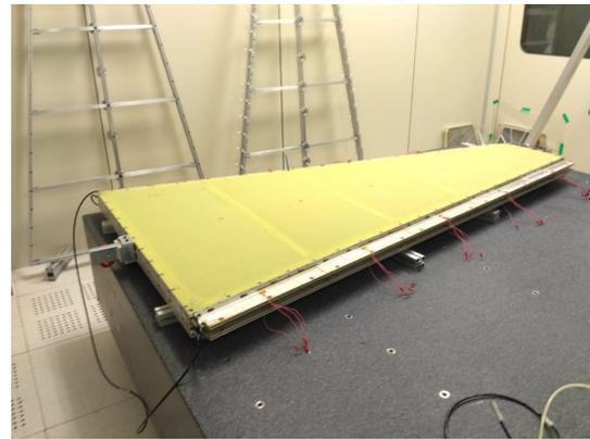
(b) Picture of one SM1 Modules on the granite plane after the construction.
