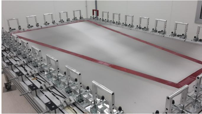
(a) Picture of one mesh during the glue curing on the transfer frame.
