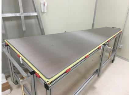
(a) Picture of one finalised drift panel at LNF. The mesh can be seen on top of the drift panel.
