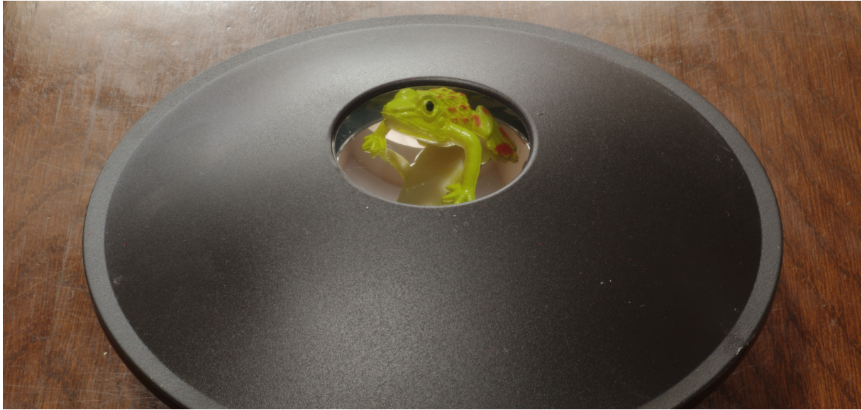
Figure 50: The “physics toy” used to get a cheap parabolic mirror. Note that the plastic frog is inside the mirror and not above.
