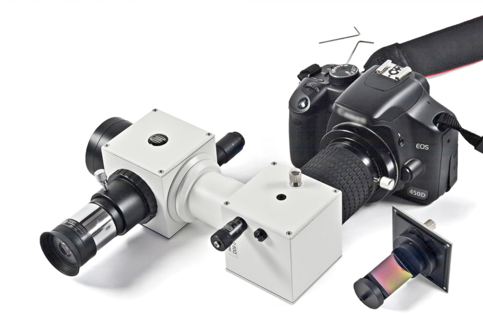
Figure 62: “DADOS Slit - Spectrograph” produced by Baader Planetarium. The light enters on left side. A special system of mirrors select light of star by a slit in a mirror in a left box and a grating separates the light by wavelength in right box.
