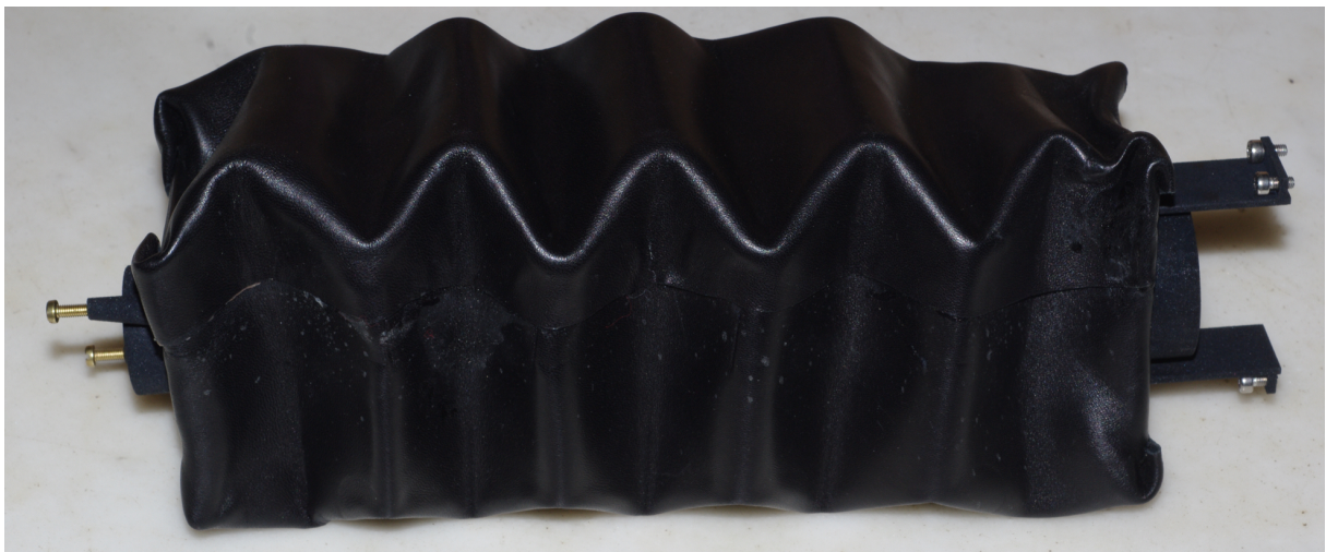
Figure 70: Photo of the bellow manually realized to interconnect the “star selection box” with the “optics box”.
