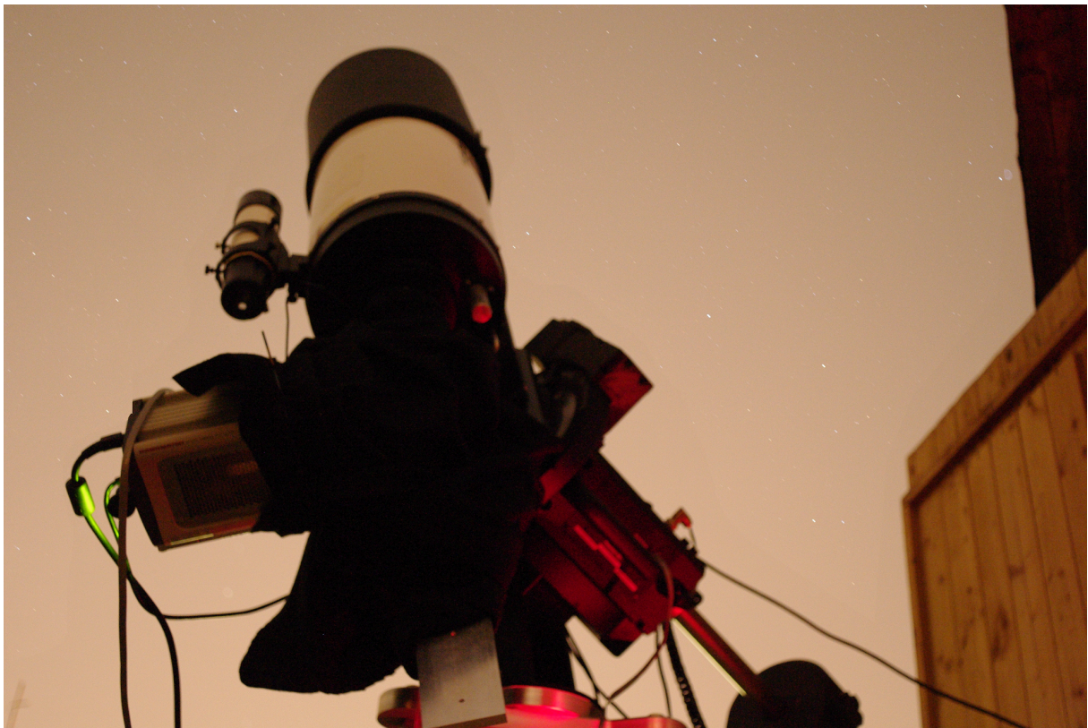
Figure 75: The prototype polarimeter connected to the telescope of RomaTre physics department, observing some stars.
