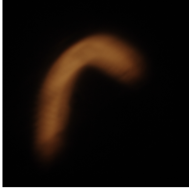
Figure 54: The photo of the collimated source at the angle of the polarization filter of 60^\circ . The original frame is cut. Final dimension is 1500 \times 1500 pixels equals to 7.5\text{mm} \times 7.5\text{mm} . The photo was acquired by reflex camera Pentax K-7 without lens. The image is the incandescent filament of the small lamp.
