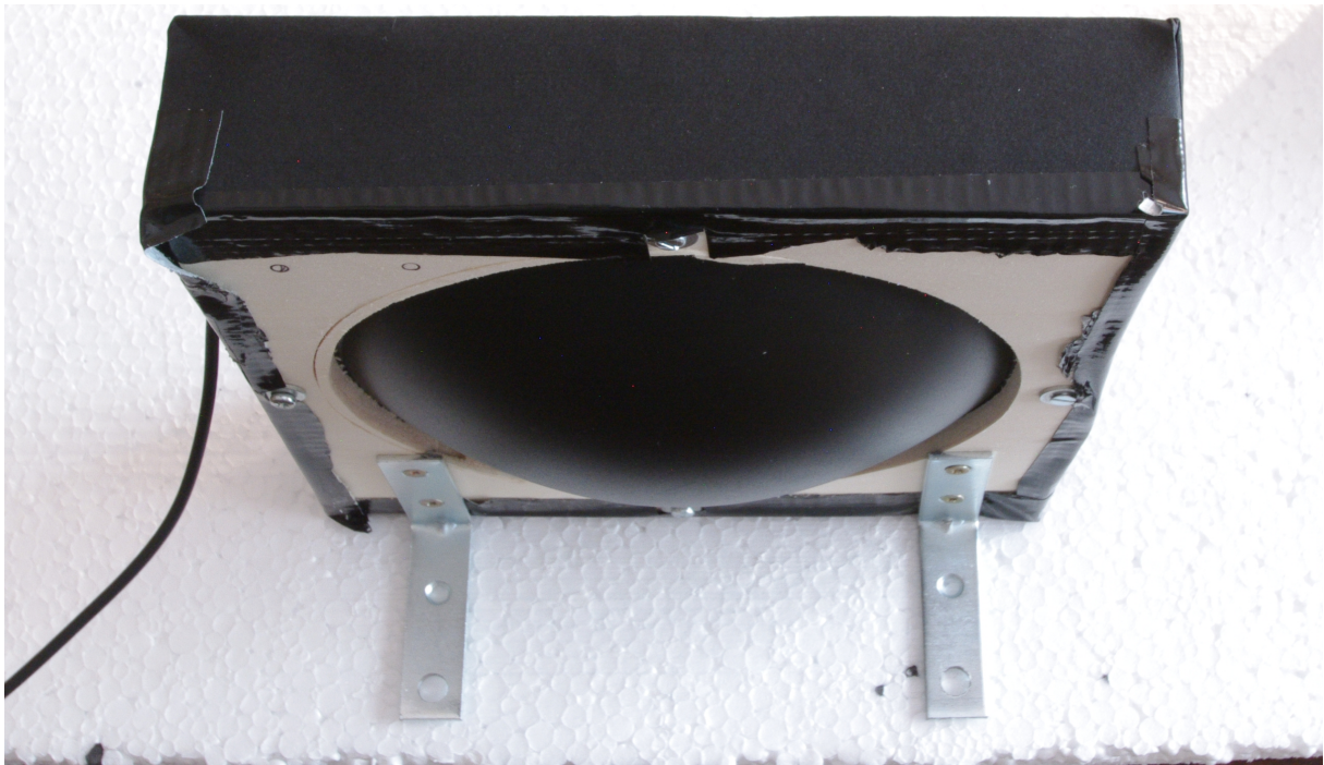
Figure 52: The collimated light source. Back view. The metallic supports to screw the source light to desk are visible.
