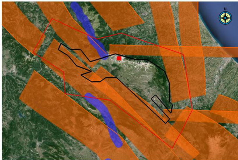
Figure 3.14: Map of central Italy (from Google Earth-CNES/Spot Image-Data SIO, NOAA, U.S. Navy, NGA, GEBCO (2013)). Composite Seismogenic Sources (orange strips), boundary of the aquifer (25 vertices black polygon) and boundary of 10 km from the edge of the aquifer (10 vertices red polygon). The red dot represents LNGS-INFN. The area under consideration is the intersection between the red polygon and the orange strips.
