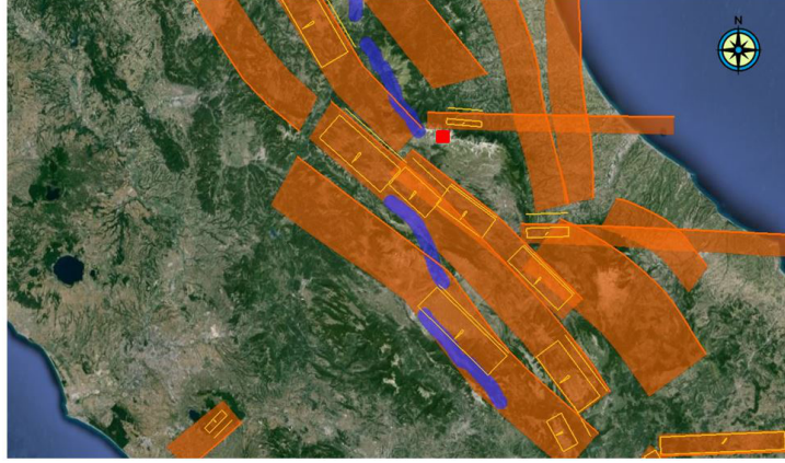
Figure 3.1: Map of central Italy (from Google Earth-CNES/Spot Image-Data SIO, NOAA, U.S. Navy, NGA, GEBCO (2013)). Individual (yellow lines), Composite (orange strips) and Debated Sources (purple bold lines) in the central Italy, based on geological and geophysical data and characterized by geometric and kinematic parameters, identified by Basili et al. (2008). The red dot represents LNGS-INFN.
