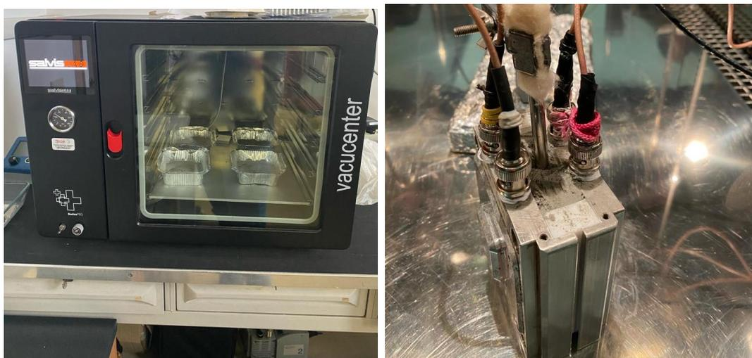
**Figure 7.4:** The dry samples were tested at varying temperature and they were placed in a vacuum oven (left panel) for 24 hours to eliminate residual moisture. On the right panel is reported the capacitive cell connected to the LCR meter and filled with dry analogue.
