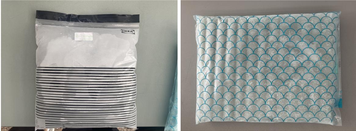
**Figure 8.4:** Icy targets used for the GPR measurements. The picture on the left is the distilled water ice target realized to replicate the ice lens. The right picture shows the ice/regolith mixture realized with frozen saturated glass beads.
