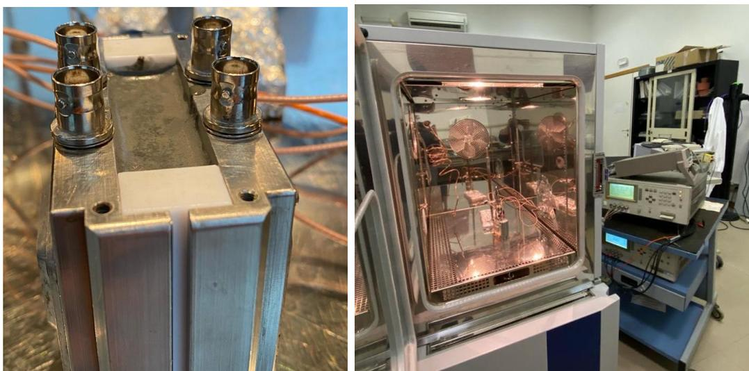
**Figure 7.5:** The left panel shows the capacitive cell filled with the saturated mixture of distilled water and regolith analogue. The right panel shows the measurement cell into the climatic chamber connected to the LCR meter.
