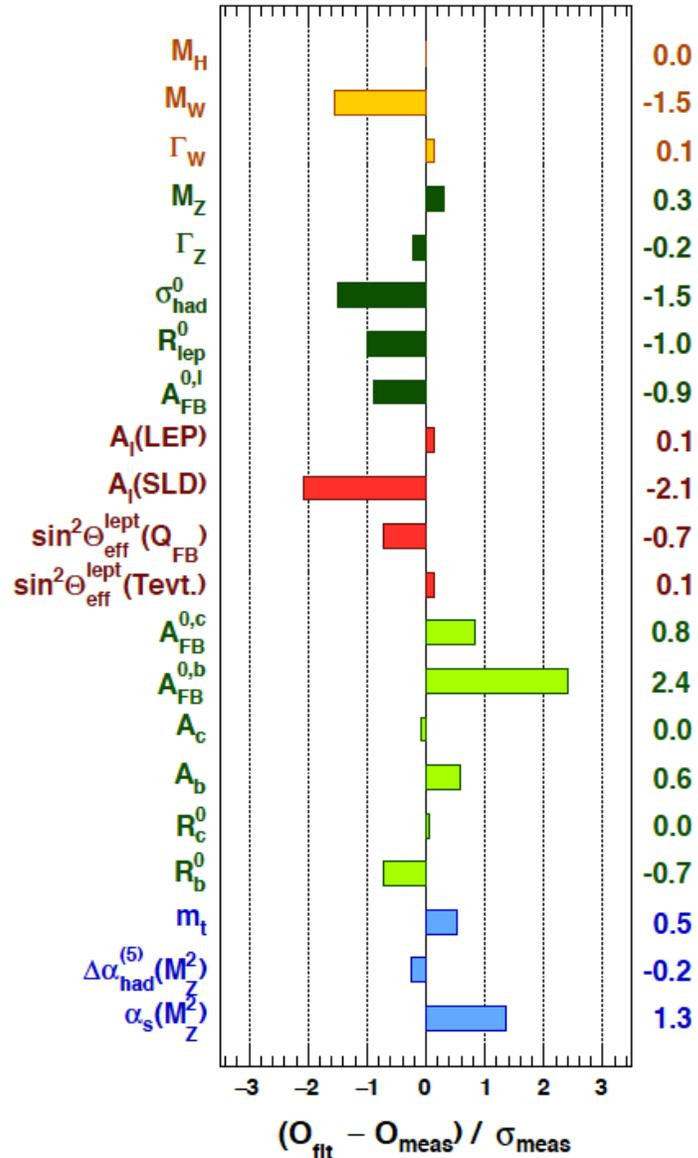
Comparison of the results with the indirect determination in units of the total uncertainty, defined as the uncertainty of the direct measurement and that of the indirect determination added in quadrature.
