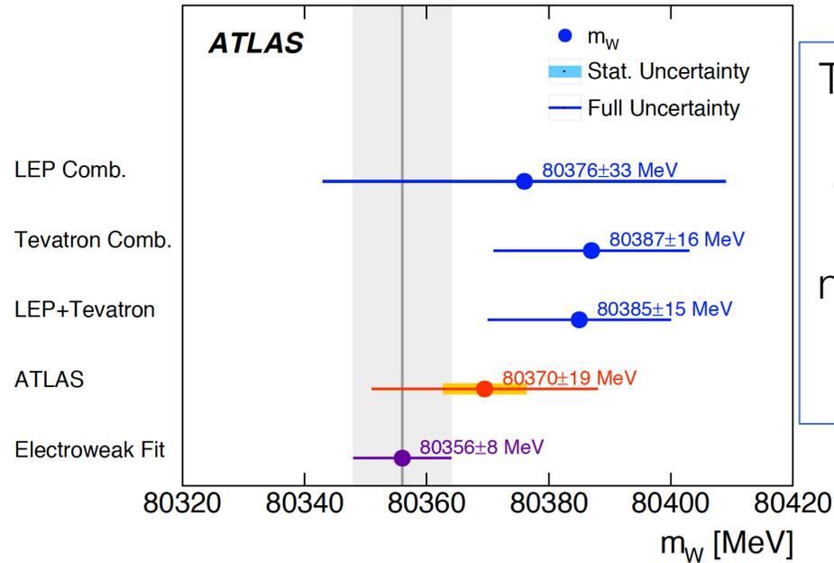
The determination of  $m_W$  from the global fit of the electroweak parameters has an uncertainty of 8 MeV  $\rightarrow$  natural target for the precision of the experimental measurement of  $m_W$ .
