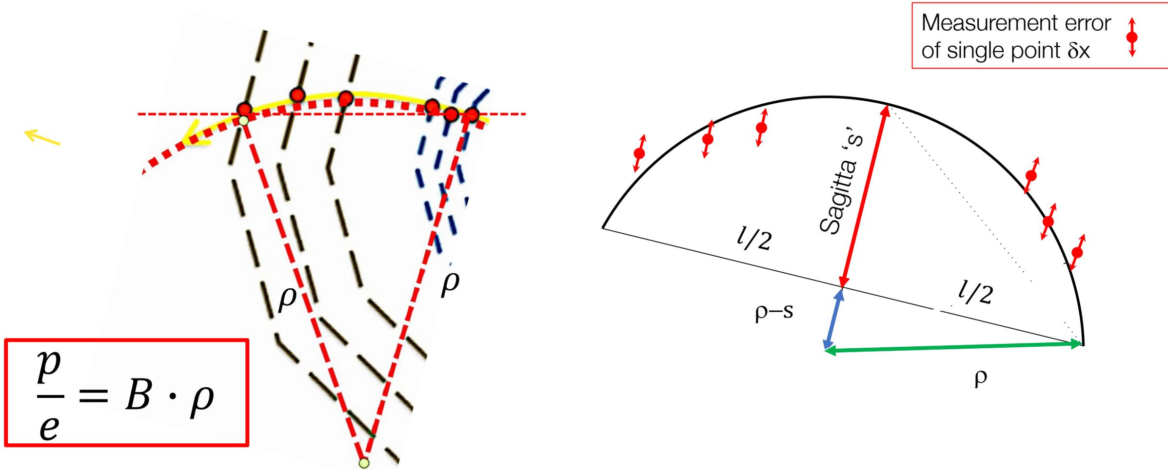
Momentum is determined by measuring the radius of curvature in magnetic field  $p \propto \frac{1}{\rho}$ .
