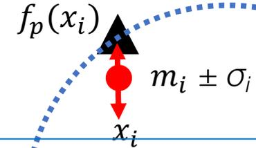
Physical meaning: distance between fit function and hit normalised to measurement error
