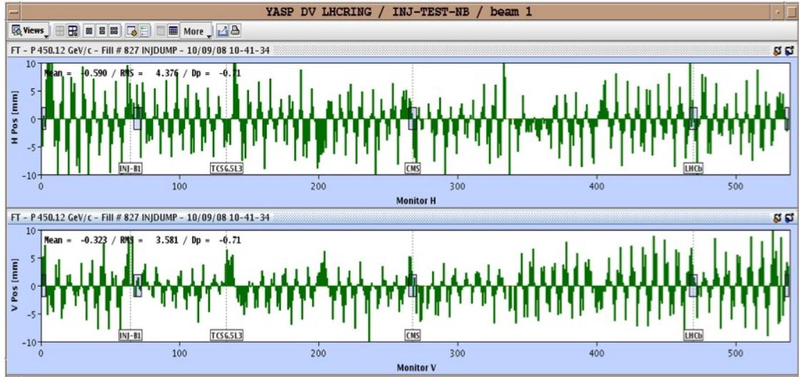
The figure on the left shows the transverse oscillations in the transverse plane of LHC as measured by the monitoring equipment **in 1 turn**. One important parameter is the the number of oscillations in the horizontal and in the vertical plane
