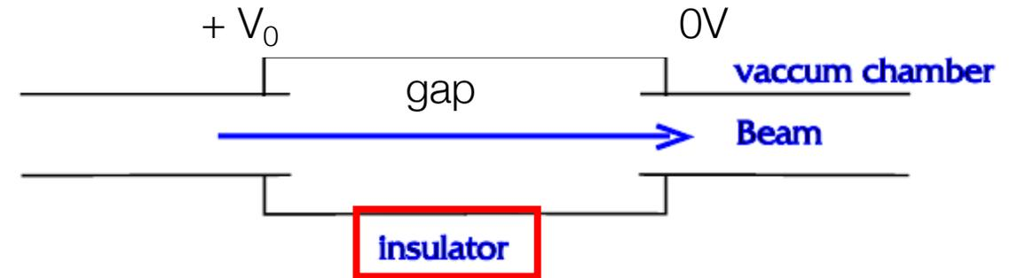
In order to accelerate the beam of particles we need a longitudinal electric field (magnetic fields cause deflections but they do not change the overall particle momentum).
