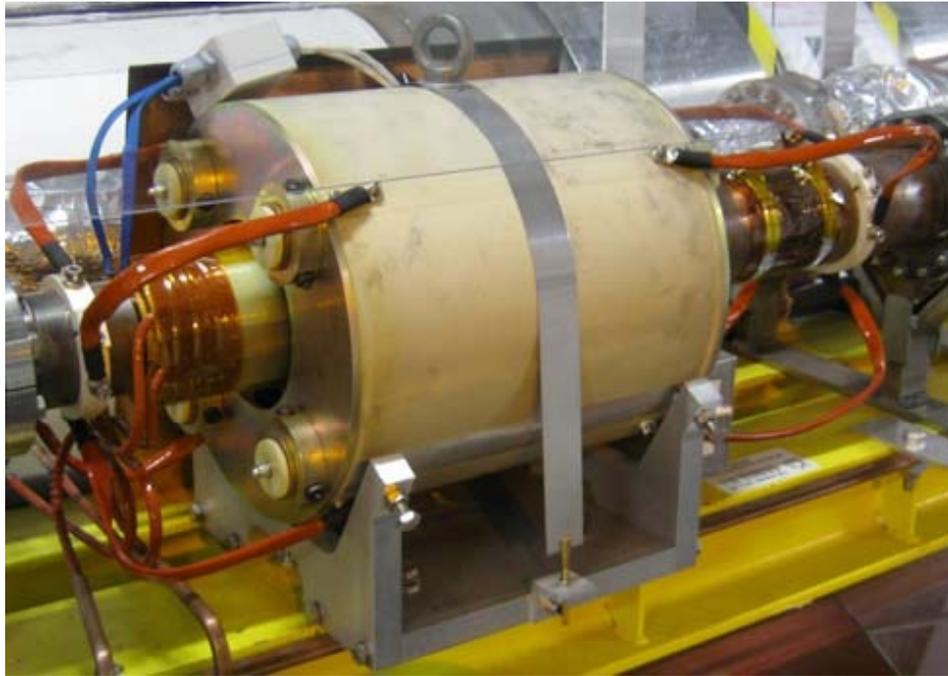
DCCT Beam Current Transformer
