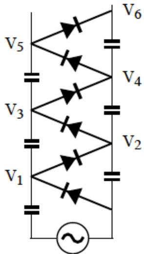
**Cockcroft and Walton:** acceleration mechanism based on a rectifier circuit, diodes and capacitors.
