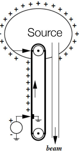
**Van de Graaff** designed a DC accelerator that used a mechanical transport system to carry charges, sprayed on a belt or chain, to a high-voltage terminal.
