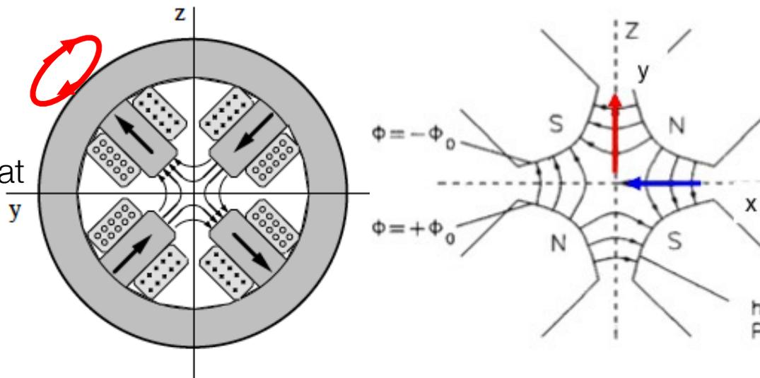
Particles travelling at the centre of the quadrupole do not experience any field and are unaffected.
