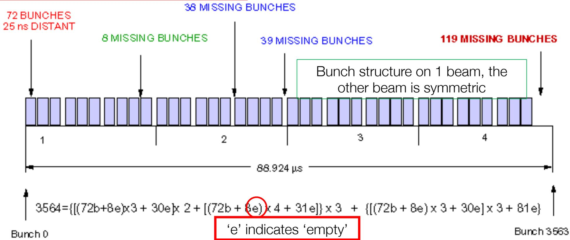
$$\text{Filled bunches} = 2808 = \{ [(72b)x3]x2 + [(72b)x4] \}x3 + \{ [(72b)x3]x3 \}$$
