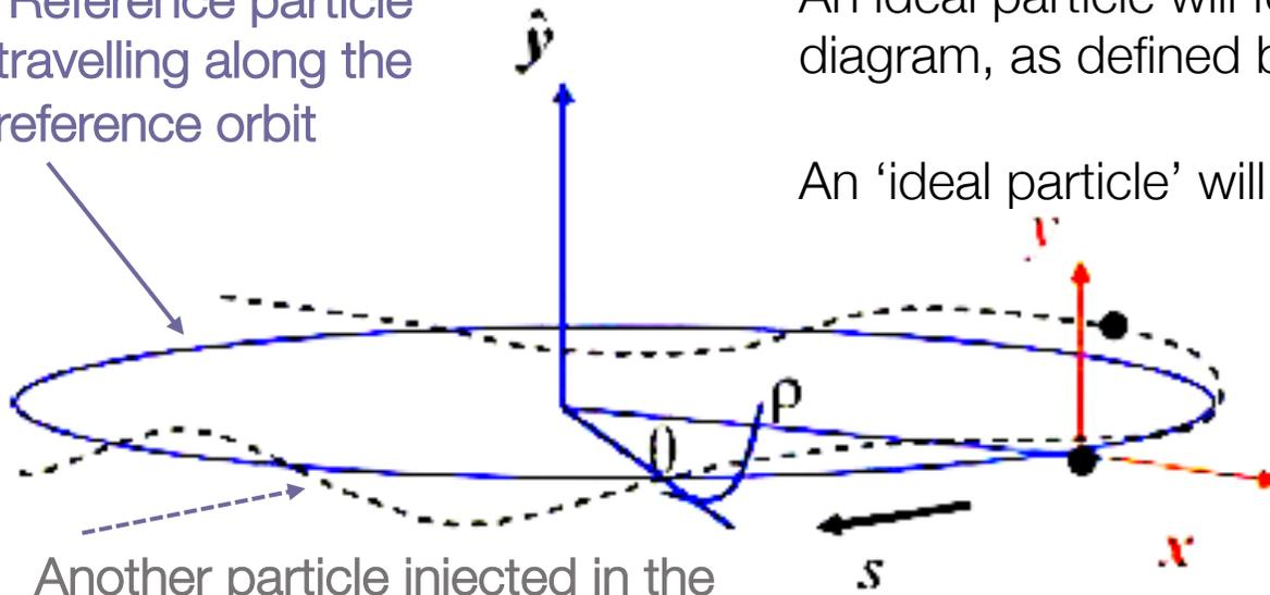
An 'ideal particle' will travel exactly along the circle (if injected exactly at the initial conditions used in the design of the accelerator, in practice injected in the horizontal plane, tangent to the circle). **Solid line**
