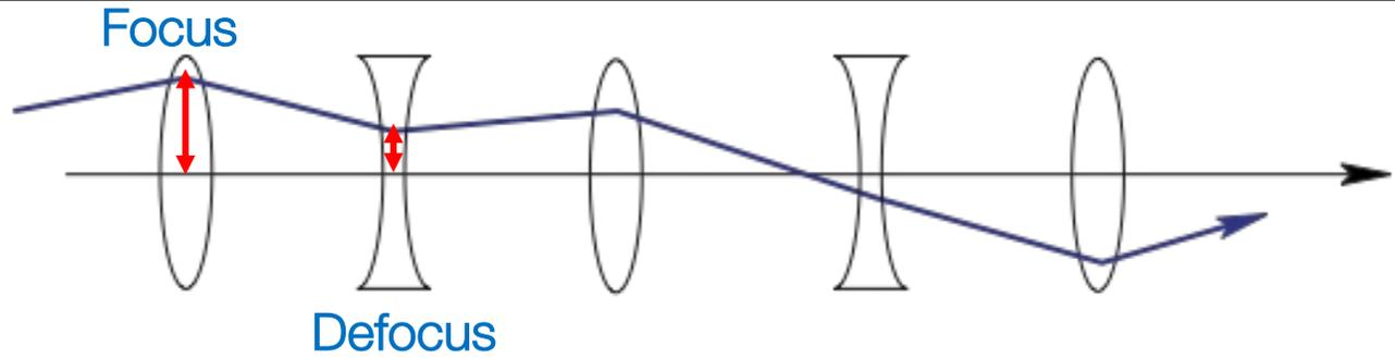
Alternating focusing and defocusing quadrupoles leads to an overall focusing:
